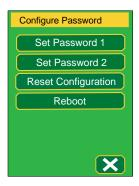
Password options are available through the Configure Passwords menu. The Password Level 1, Password Level 2, and Reset to Factory Settings options are described below. The Reboot option will force the monitor to shut down and then restart.
