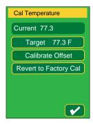
This screen is available only on models with the optional temperature humidity sensor and after the level 2 password has been entered. This feature allows the monitor to be installed in an area that is known to be characteristically cooler or warmer than the rest of the space (e.g., near a photocopier). This requires that a desired value ("target temperature") be entered.
