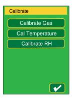
Calibration procedures are initiated at the Calibrate menu. Refer to local regulations for calibration requirements. Calibrate the monitor at least once a year to maintain the highest level of accuracy.
