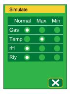
Simulated output permits creating high or low outputs on the three sensors, allowing the operator to verify that the system will respond as planned to changes in the gas level, temperature, or humidity level. Any combination of minimum, maximum, or normal values of gas, temperature, and humidty can be simulated. Default simulation selections are normal for all three parameters.
