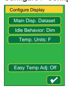
Temp Units is available only for monitors with temperature/humidity sensors. Easy Temp Adj is available for digital monitors and those fitted with temperature/humidity sensors.
