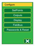
The monitor's customization begins with the Configure menu. The setpoints option is available only with digital monitors and monitors equipped with relays. The fieldbus option is available only with digital monitors.
