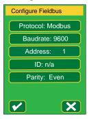
This screen is available only on models with the BACnet/Modbus interface. The monitor's fieldbus configuration options apply only to RS-485-enabled units. The monitor will reboot whenever the [Accept] button is pressed so that the new communication parameters will be implemented correctly.
