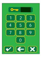
The user's password, a four-digit number, is entered by pressing the appropriate numbers on the touchscreen. As each number is selected, it is shown near the top of the display. After the four numbers are displayed, press  $[\checkmark]$  to proceed to the main menu. Press  $[\leftarrow]$  to delete the last digit entered (repeat to delete more digits). Press  $[\times]$  to return to the Default Display screen without entering a password.
