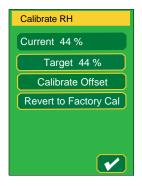
This screen is available only on models with the optional temperature humidity sensor and only after the level-2 password has been entered. The monitor is precalibrated so calibration is not necessary.
